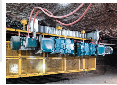
Alignment-Free Belt Drive underground roof/"back" mount setup
