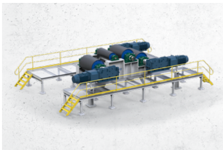
Triple 450HP Alignment-Free Conveyor + Catwalks
