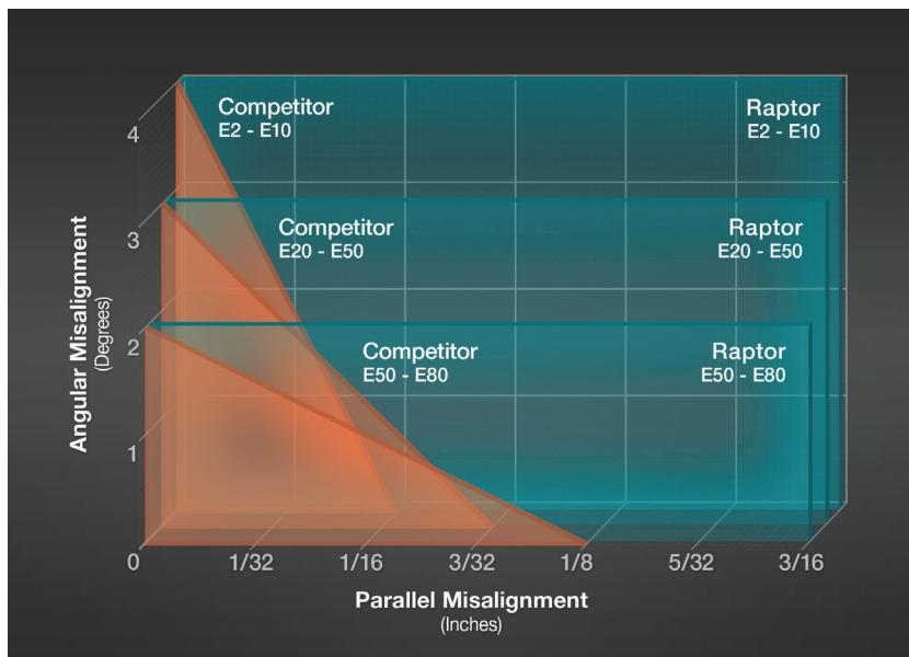
The Raptor provides accommodation of shaft misalignment during installation, operation, and replacement better than competitive urethane elements.
