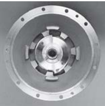
Internally mounted, oil lubricated backstops are available for all Planetgear 7000 reducers. Backstops are not limited by load, duration, or frequency of operation. They can operate in extreme pressure oil, and can be installed in the field without removal of gearing.
